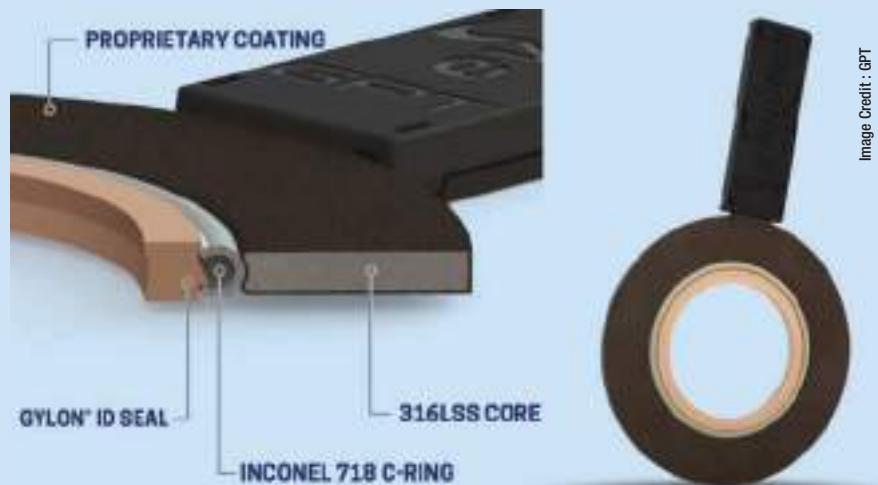
EVOLUTION, the fully-coated isolation gasket.
