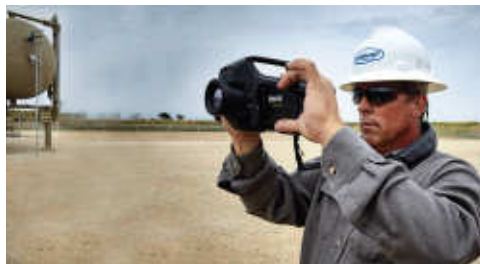
OGI cameras can be used to detect methane and other hydrocarbon emissions.
