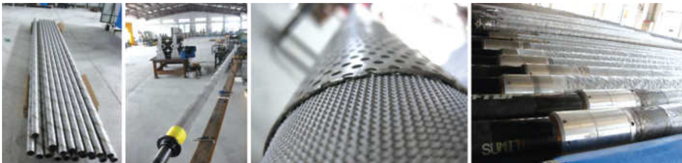
The 7m jackets (left to right) are fitted with layers of the premium mesh screen jacket with an outer shroud on the outside and a drainage layer underneath.
