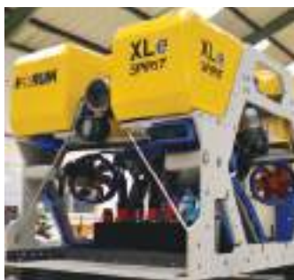
The XLe Spirit can maximise its stability for use as a sensor platform.
