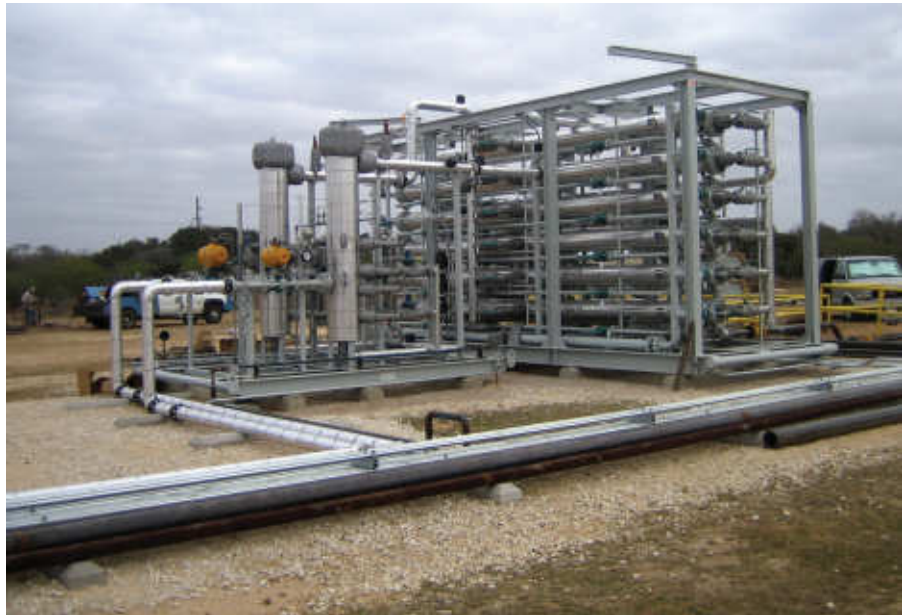
Figure 2: A new process for CO 2 removal for natural gas will be discussed.
