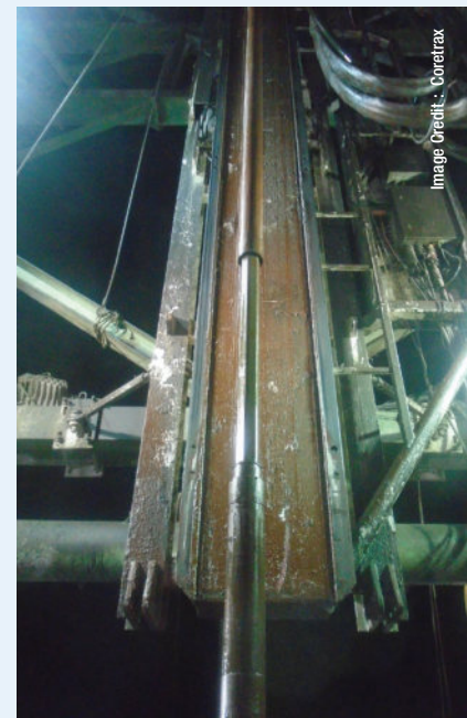
Figure 2: The BHA design and placement of the bumper subs allowed for optimum placement of the LTTT-HD and subsequent testing of both liner tops in a single trip.
