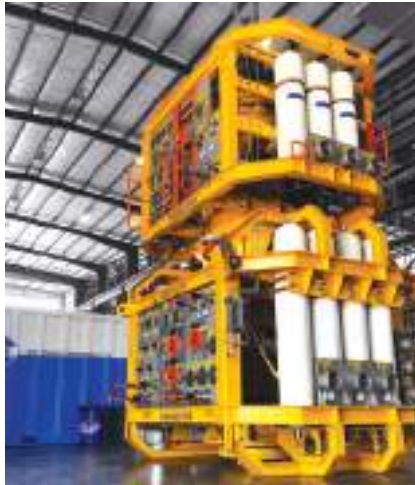
Trident's well control package (WCP) is built around the reliable shear/seal design of the Interventek Revolution valves.
