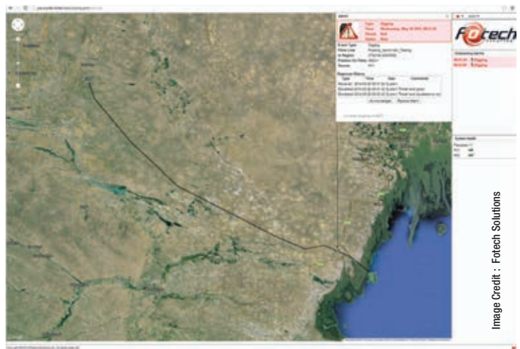
Using DAS technology, disturbances are detected and an alarm raised.
