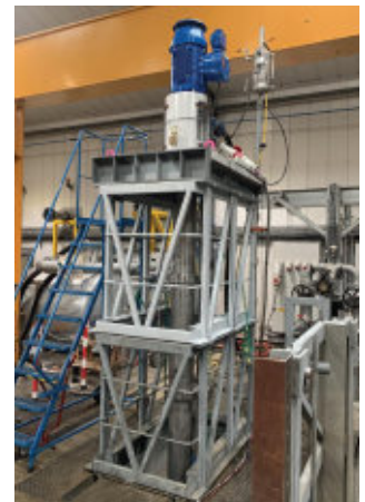
Amarinth API 610 VS4 vertical pump undergoing final test before delivery.
