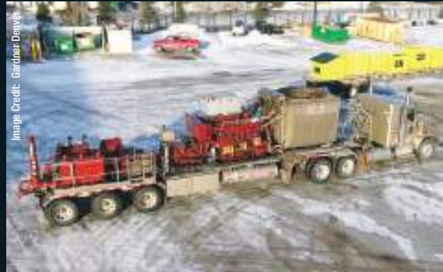
Gardner Denver's new Thunder 5000 HP Quintuplex pump at STEP energy services field trial.
